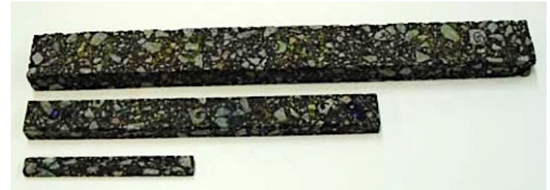
Figure: 1x, 2x, and 3x asphalt mixture beam specimens (Marasteanu et. al., 2009)
