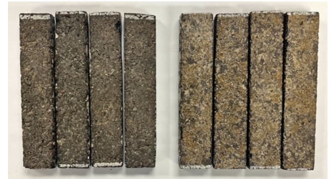
Figure: Modified BBR beams (127 mm × 25.4 mm × 12.7 mm)
