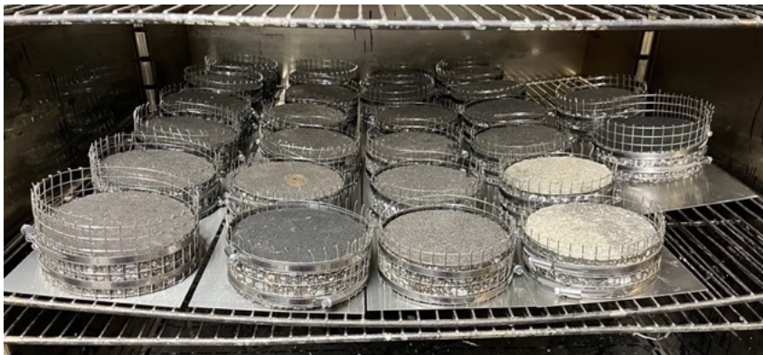
Cores placed in an oven for lab aging
