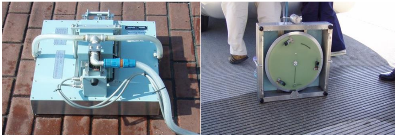
FIGURE 2-2: Dynamic Friction Tester, ASTM E1911
