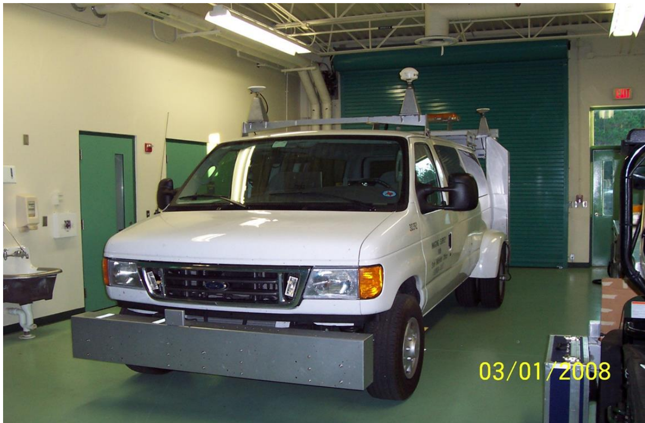
FIGURE 3-1: Photo of FDOT Multi-Purpose Survey Vehicle (MPSV)
